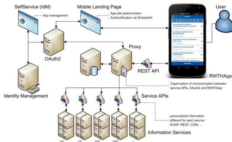
**Figure 1** Architecture overview of the infrastructure to access data from existing systems.
